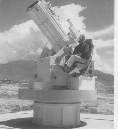
through shake-down tests in Albuquerque, is operated here by Joel 5224). control stick in his hand "electronic memory" which tracks objects almost automatically.
